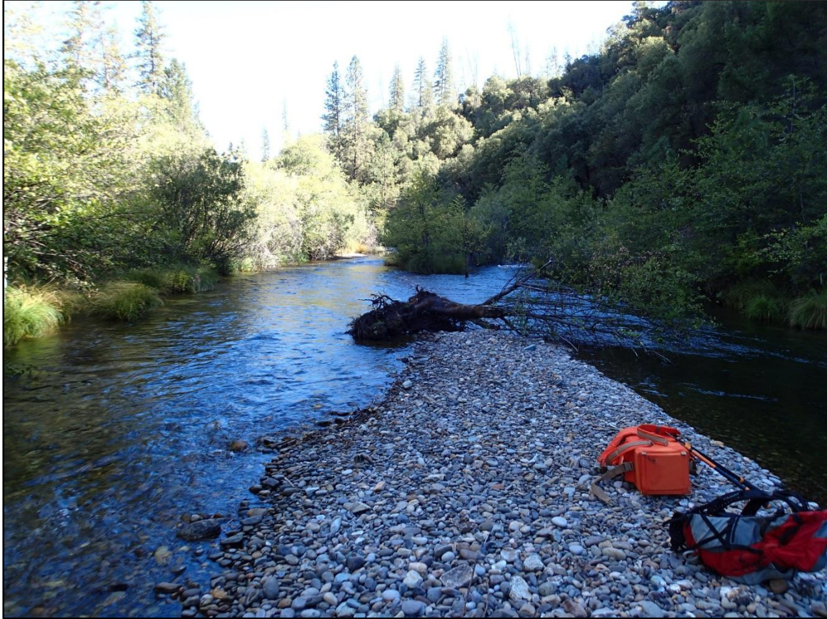
Figure 22. Upstream view from the 2013 leading edge 1,200 feet downstream of the Below Dog injection site. Note the complex form of the lateral bar/riffle migrating through the bedrock pool: high velocity gravel bed on the left side photo; deep, slow bedrock/boulder pool on the right side; riparian disturbance (uprooted alder); transverse flow across the bar. The alignment and trajectory is keyed to the mid-channel bedrock island at the top of the photo (~75 cfs).
