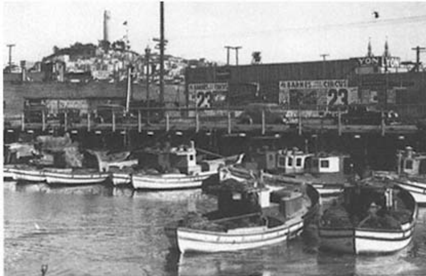
Monterey. The boats pictured in the 1930s at Fishermen's Wharf, San Francisco, were powered by one-cylinder gasoline engines. The Monterey replaced the sail-powered felucca in the California commercial salmon fishery. (National Maritime Museum)
