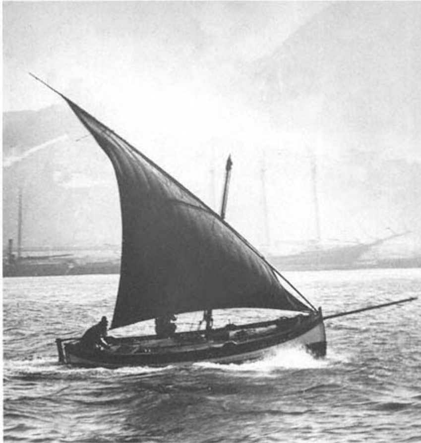
Lateen-rigged felucca, a type of fishing boat used by early Italian, and to some extent Portuguese and Greek, fishermen on San Francisco Bay. (National Maritime Museum)
