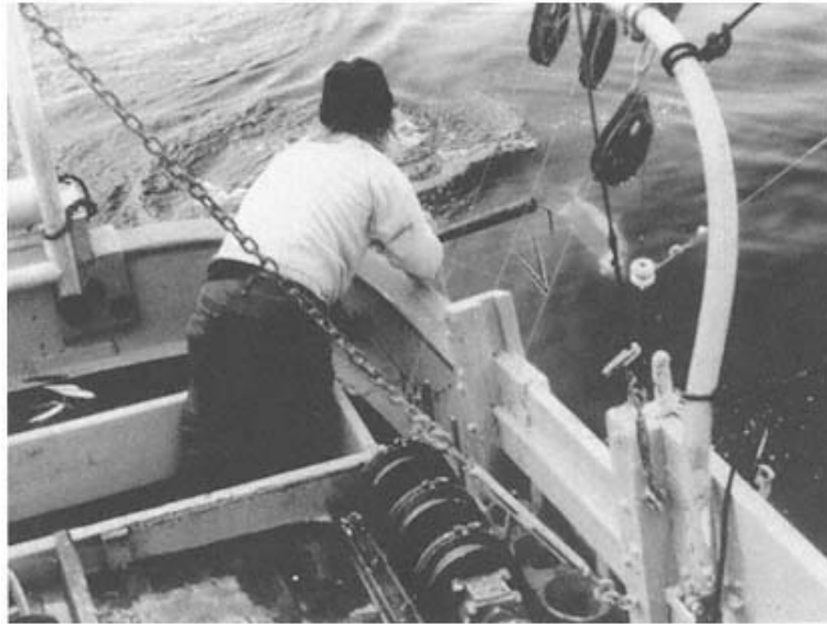
Commercial salmon troller preparing to land hooked salmon. Note power winches (gurdies) that raise and lower troll lines.
