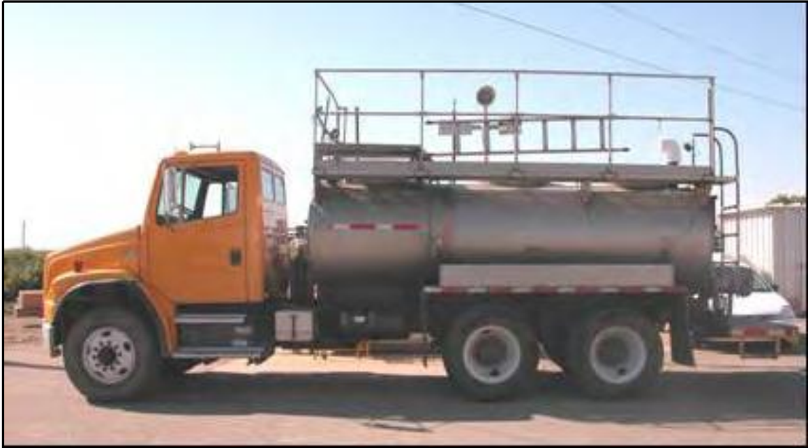
FIGURE 3.—The Tracy Fish Collection Facility fish-hauling truck. The tank is cylindrical in shape, 1.2 meters (4 feet) deep, 4.4 meters (14.4 feet) long.
