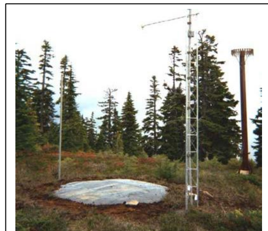
A typical snowpack telemetry site includes a snow pillow, an antenna with solar panels and a temperature sensor, and a precipitation gauge (brown structure in background, right)
