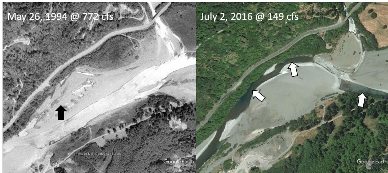
Figure 2. Changes at Freeman extraction location on the Chetco River at the Confluence of North Fork Chetco River between 1994 and 2016. Filled arrows indicate isolated pools, open arrows indicate connected deep pools (Google Earth 2018).
