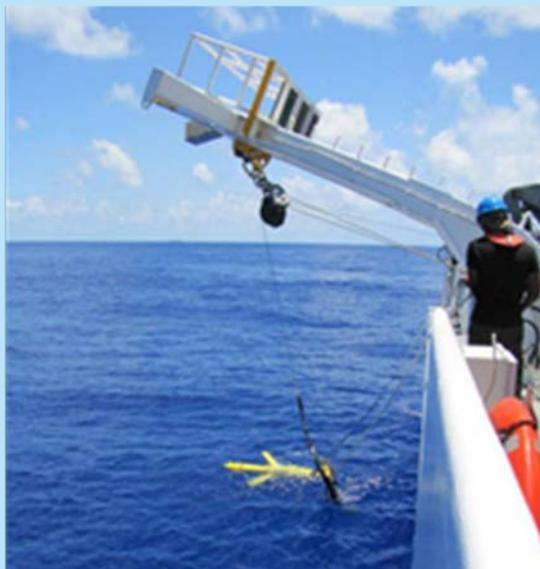
**Figure 3.1.** An unmanned underwater vehicle (UUV) is deployed from a Naval Oceanographic Office (NAVOCEANO) survey vessel. (Image courtesy of U.S. Navy)
