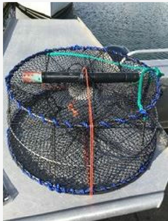
Smart dissolved oxygen sensor deployed on spot prawn traps by Washington Department of Fish and Wildlife (WADFW) managers as part of the Puget Sound pre-season fishery survey. Credit Washington DFW.
