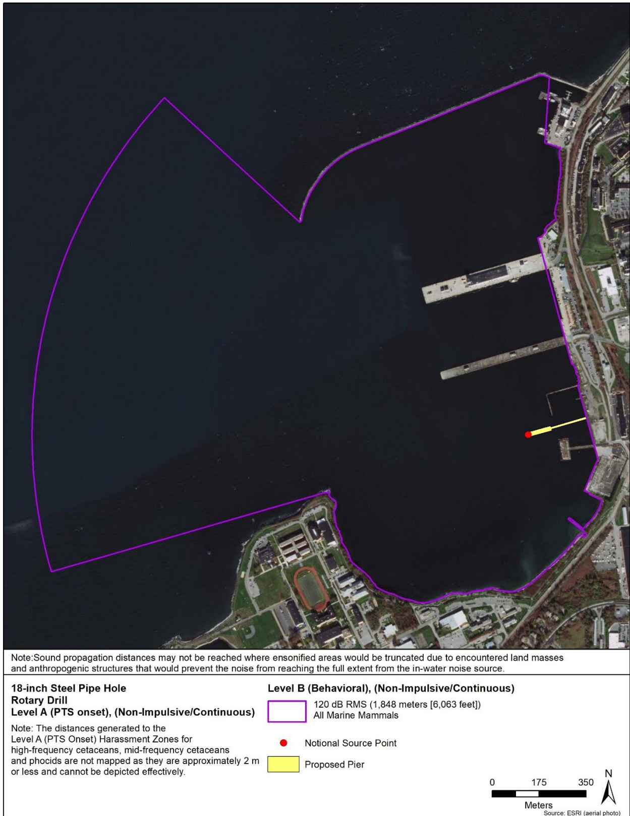
Figure 6-15 Level B (Behavioral) Harassment Zone from Rotary Drilling Activity at the Trestle (Bents 1-18) – Hole for 18-inch Steel Pipe
