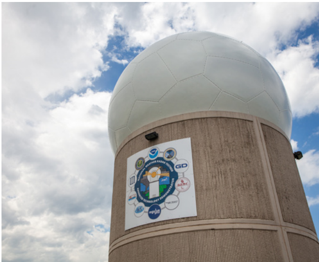
Installed at the National Weather Radar Testbed facility, the Advanced Technology Demonstrator is the first full-scale, S-band, dual-polarization Phased Array Radar built from the ground up and designed specifically for use as a weather radar.
