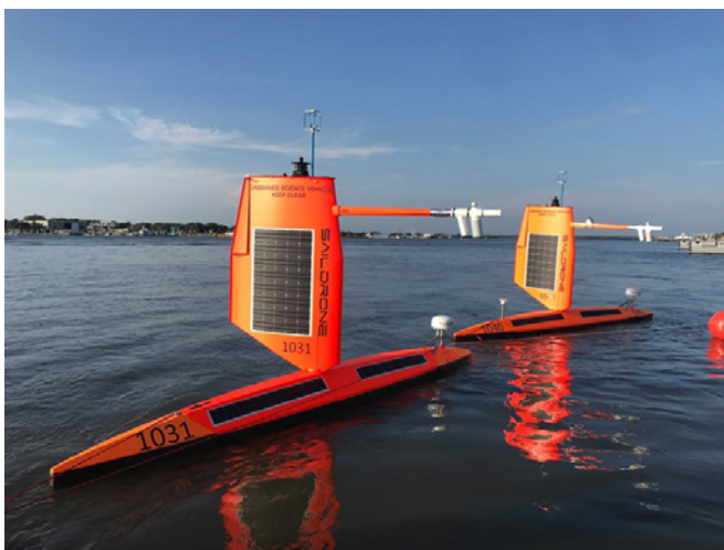
NOAA and Saildrone launched the uncrewed surface vehicles from Jacksonville, Florida at the beginning of the 2021 Hurricane Season to track storms and collect data to improve forecast models. Credit Saildrone
