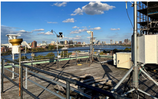
Over the past 8 years samples of methane and carbon dioxide captured at this urban observatory on the roof of a Boston University building have helped scientists show that natural gas leaks from the city are much larger than previously thought. Credit: L.R. Hutya, Boston University
